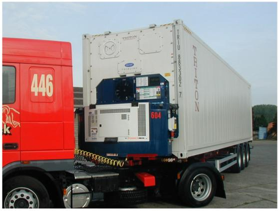
Auxiliary diesel generator unit (genset) providing power to the reefer during transport on a truck, ship or train (http://www.gopixpic.com/600/reefer-container-gensets-40kva-keyword-/, accessed 20141031).
